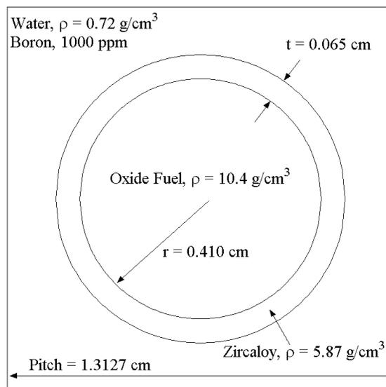
Figure 3. Unit Cell Used in Benchmark and Demonstration
