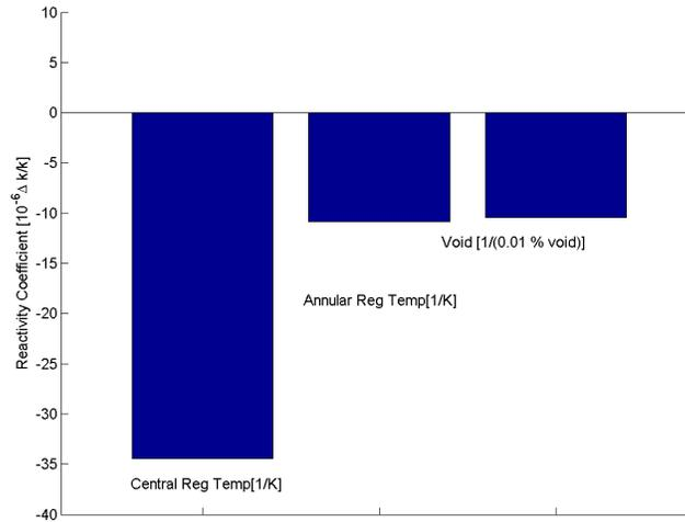
Figure 7. Reactivity Coefficients for Fresh Fuel Composition
