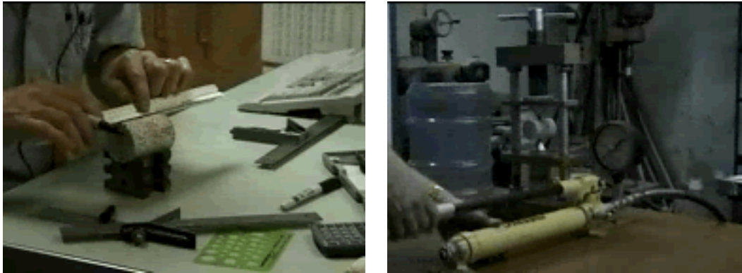
Figure 2. Procedure for a point load test. a) sample preparation, b) testing
