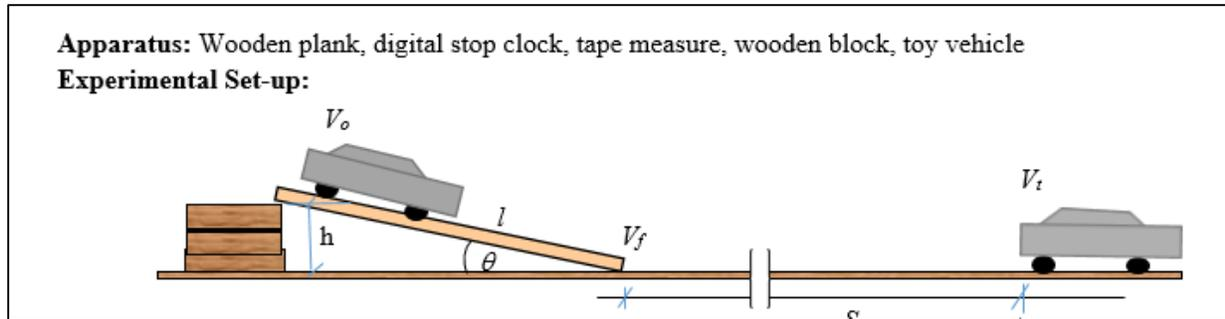
**Figure 1: Experimental set-up for project 1**
