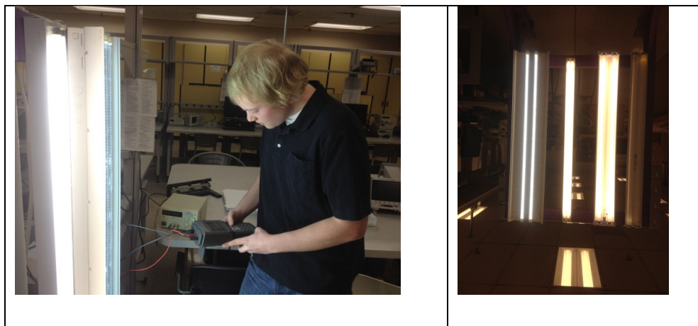
Figure 1. A custom designed and built testbed for incandescent, CFL, florescent, and LED sources for investigating harmonics studies.
