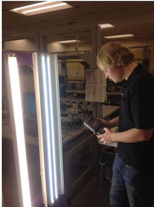
Figure 3. Very low harmonics measured when an LED tube was tested.
