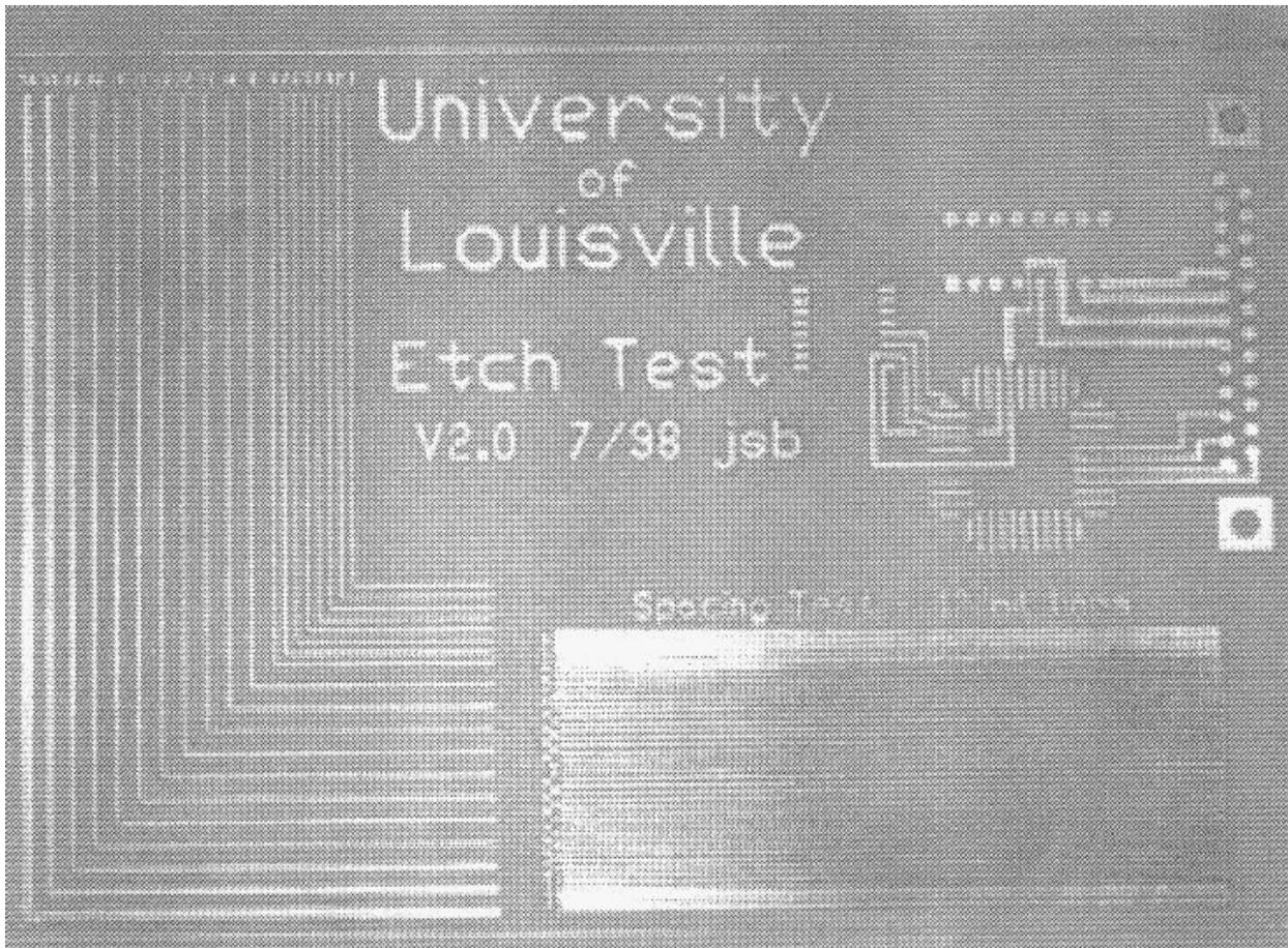
Fig. 2. Test pattern PCB after copper etching and resist cleanup.
