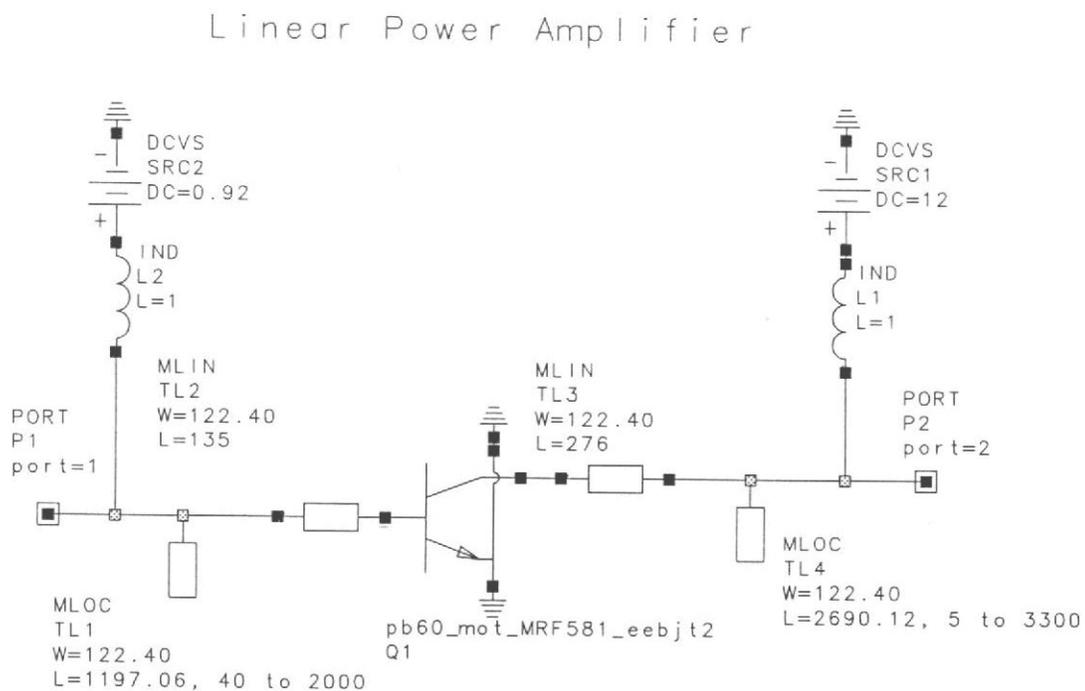
Figure 5. Schematic of Cellular Band Power Amplifier Design.
