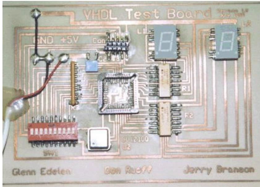
Fig. 4. Picture of the final ALU test board without the CPLD in the socket.
