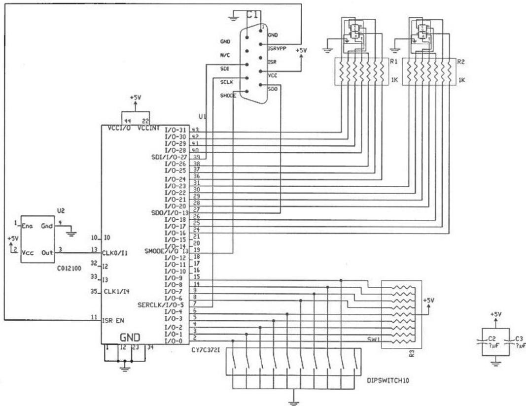
Figure 3. Schematic of the CPLD-ALU demonstration PCB.
