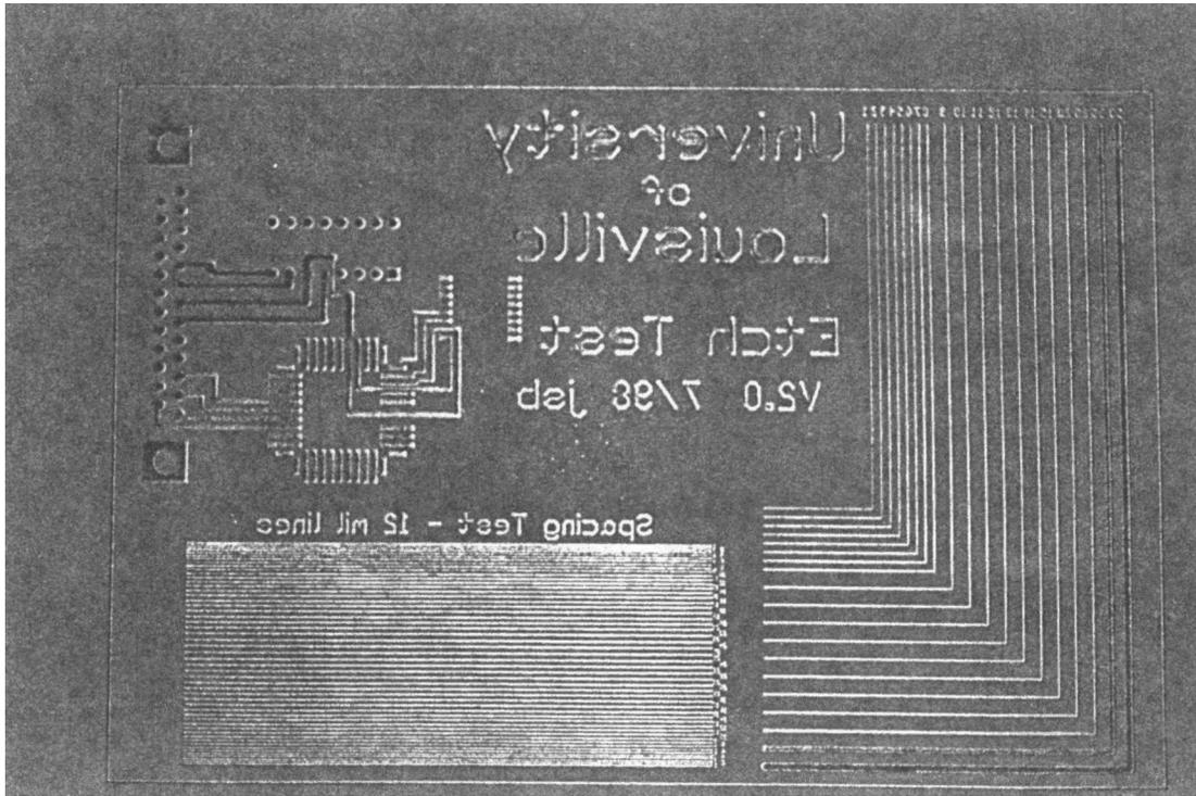
Fig. 1. PnP-Blue plotter paper test pattern mask after being fed through the laser printer.
