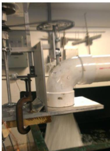
**Figure 2 - Headstock, turbine, transmission system, and PMG for the hydroelectric generator plant.**
