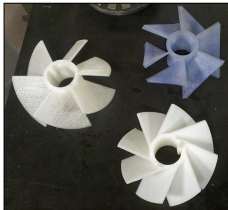
**Figure 3 - Three Kaplan turbine designs for the hydroelectric generator plant.**
