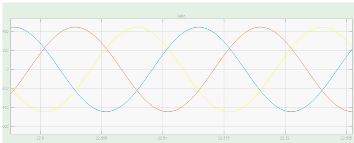
Figure 8: Three-phase bus voltages
