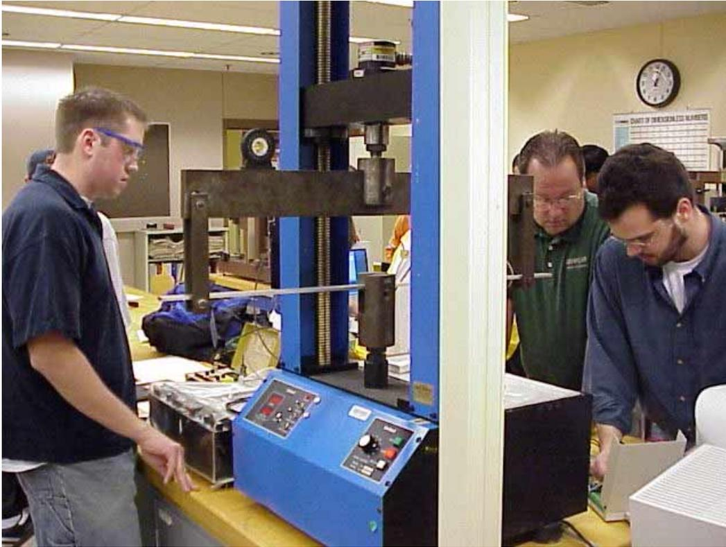
Figure 8: DAQ Calibration at the Signal Conditioning Unit
