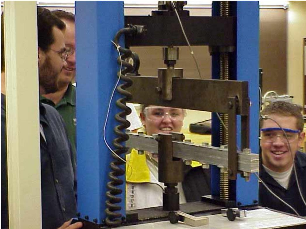
Figure 1: Three-Point Bending Set-up
