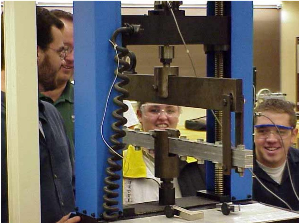
Figure 1: Three-Point Bending Set-up
