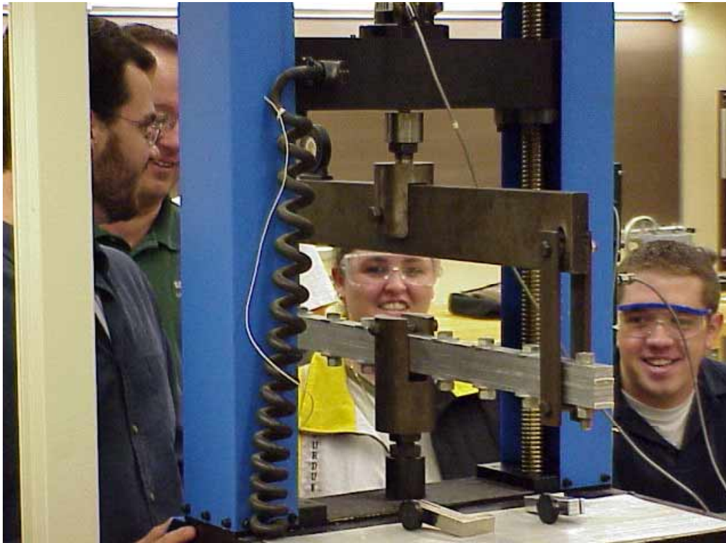
Figure 1: Three-Point Bending Set-up
