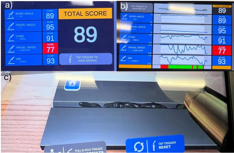
Figure 12: Butt Joint, a) Good Score, b) Score Visualizations, c) AR welded joint
