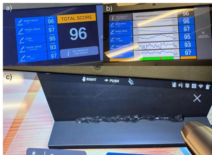
Figure 6: Tee Joint, a) Good Score, b) Score Visualizations, c) AR welded joint
