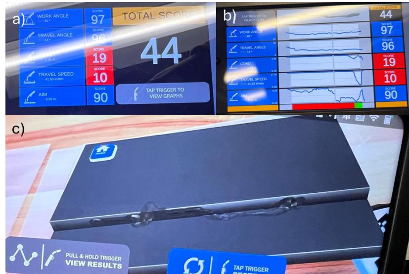
Figure 7: Lap Joint, a) Bad Score, b) Score Visualizations, c) AR welded joint
