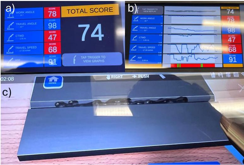
Figure 11: Butt Joint, a) Decent Score, b) Score Visualizations, c) AR welded joint
