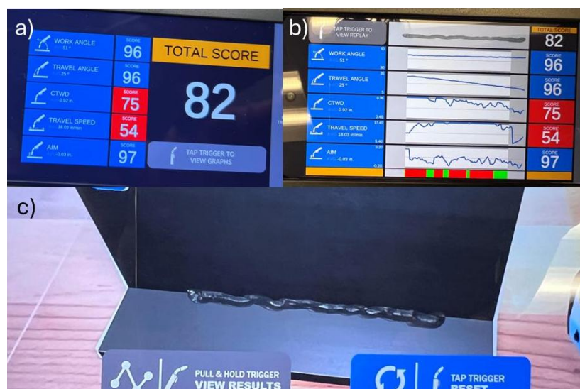
Figure 5: Tee Joint, a) Decent Score, b) Score Visualizations, c) AR welded joint
