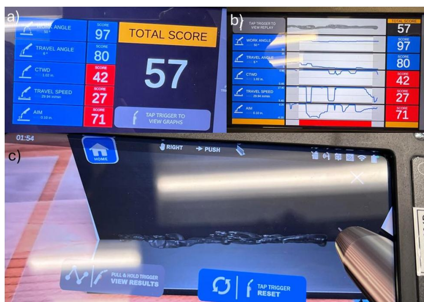
Figure 4: Tee Joint, a) Bad Score, b) Score Visualizations, c) AR welded joint
