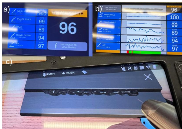
Figure 9: Lap Joint, a) Good Score, b) Score Visualizations, c) AR welded joint
