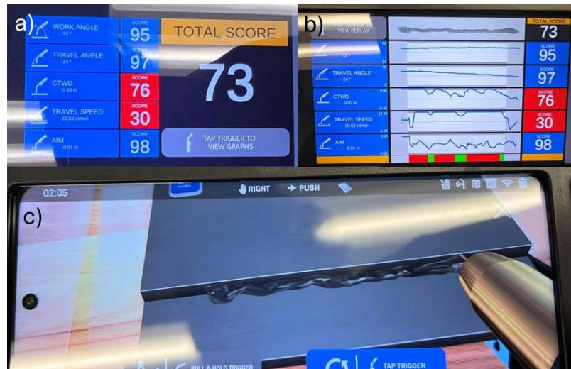
Figure 8: Lap Joint, a) Decent Score, b) Score Visualizations, c) AR welded joint
