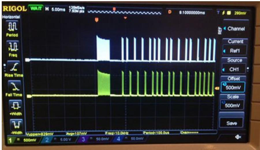
**Figure 3:** Codes generated by a TV remote control
