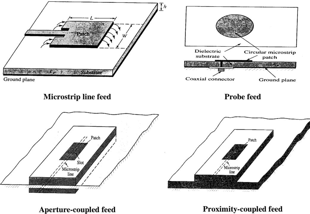
Figure 1: Typical Feed Methods for Microstrip Antennas
