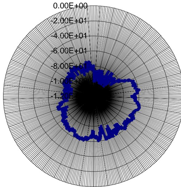
Figure 8: 2-D Polar Plot of 3GHz Patch Antenna
