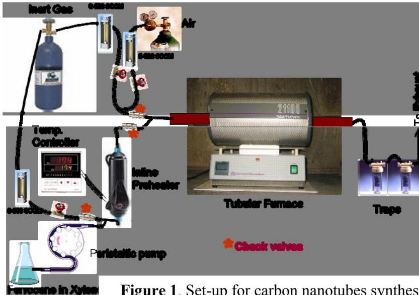
**Figure 1.** Set-up for carbon nanotubes synthesis
