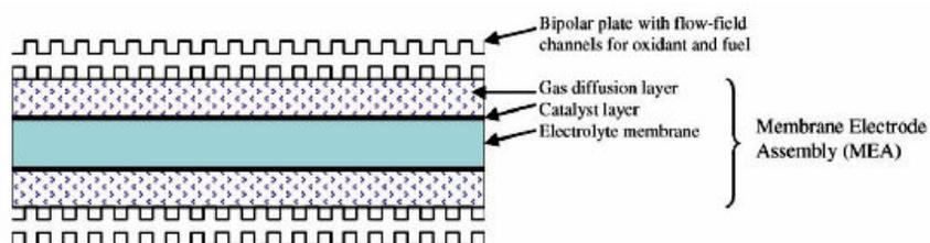
Figure 5. General Schematic representation of Polymer Electrolyte Membrane Fuel Cell.
