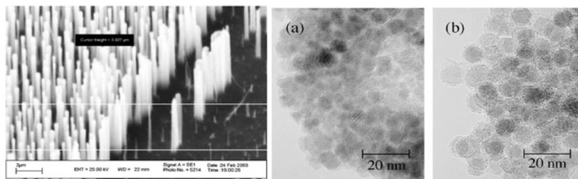
Figure 3. SEM image of a silicon anode having a nano pillar surface morphology<sup>6</sup>.
