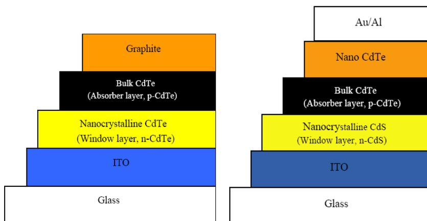
Figure 6. Device configurations of a Glass/ITO/n-Nano-CdTe/p-bulk CdTe/graphite and a glass/ITO/n-nano-CdS/p-bulk CdTe/nano-CdTe/Au solar cells<sup>13</sup>.
