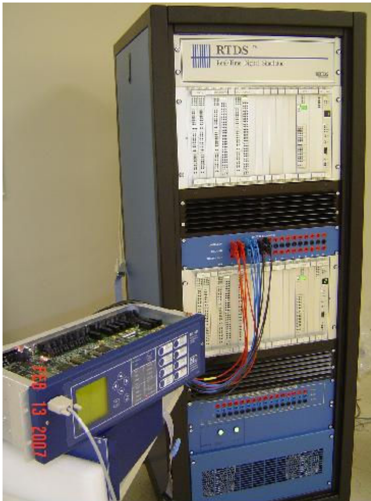
Figure 1: Actual hardware setup with RTDS for real time Hardware in the Loop test
