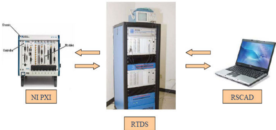
Figure 4. Setup for closed loop controller testing with RTDS
