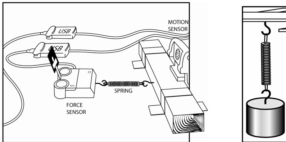
Figures 1 and 2: Determining a Spring Constant—Sensor and Non-Sensor Laboratories.
