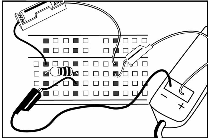
Figure 10. Measuring current in the circuits lab.
