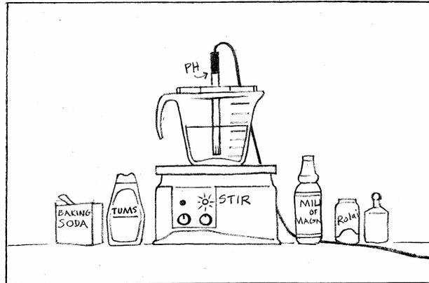
Figure 5. Measuring antacid response.
