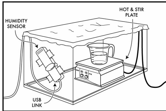
Figure 7. Taking humidity measurements.
