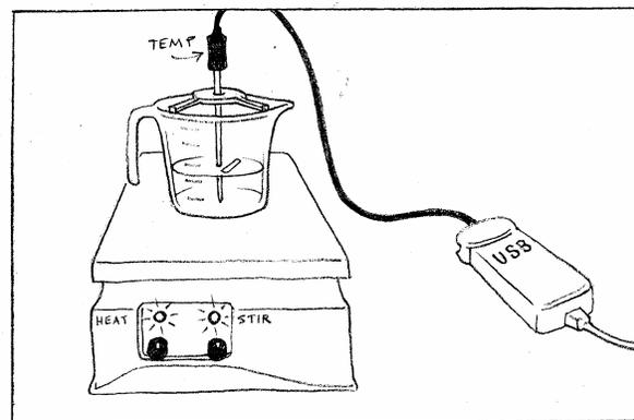
Figure 3. Temperature probe setup.
