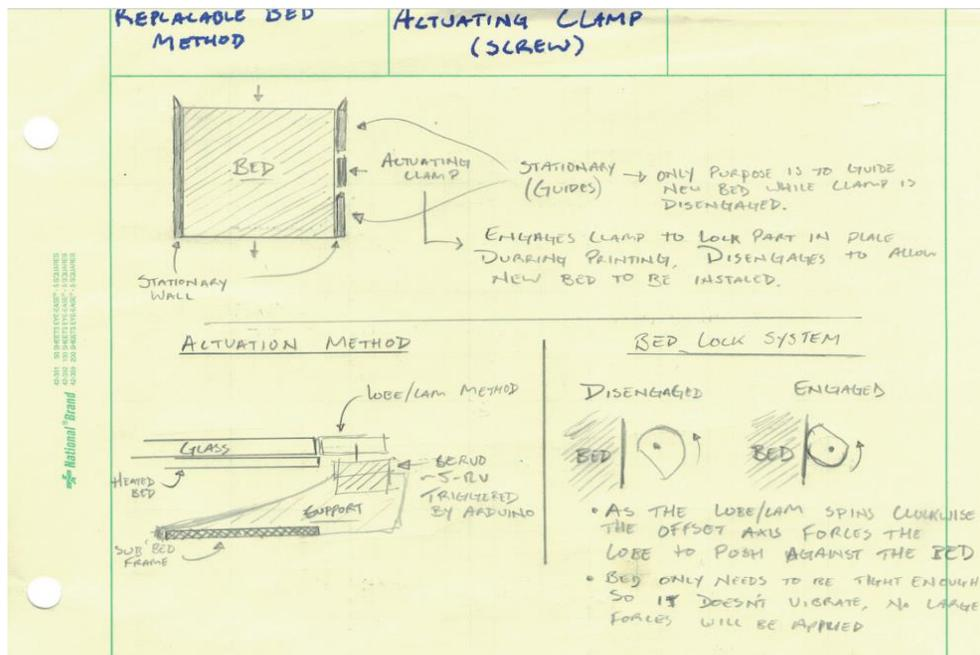
Figure 3: Initial Idea of the Cam Locking Mechanism
