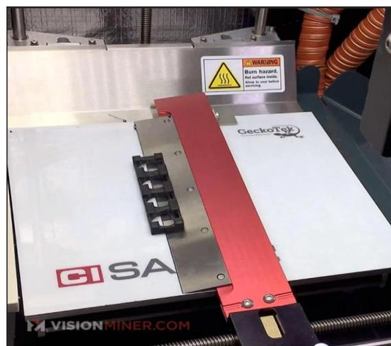
Figure 2: SAAM Part Ejection System [16]
