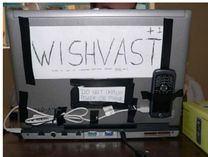
Figure 2: The WishVast hardware: one laptop, one cell phone, one USB tether.
