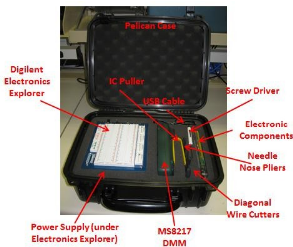
Figure 2: Portable electronics self-contained lab components utilizing the Electronics Explorer™ Board.
