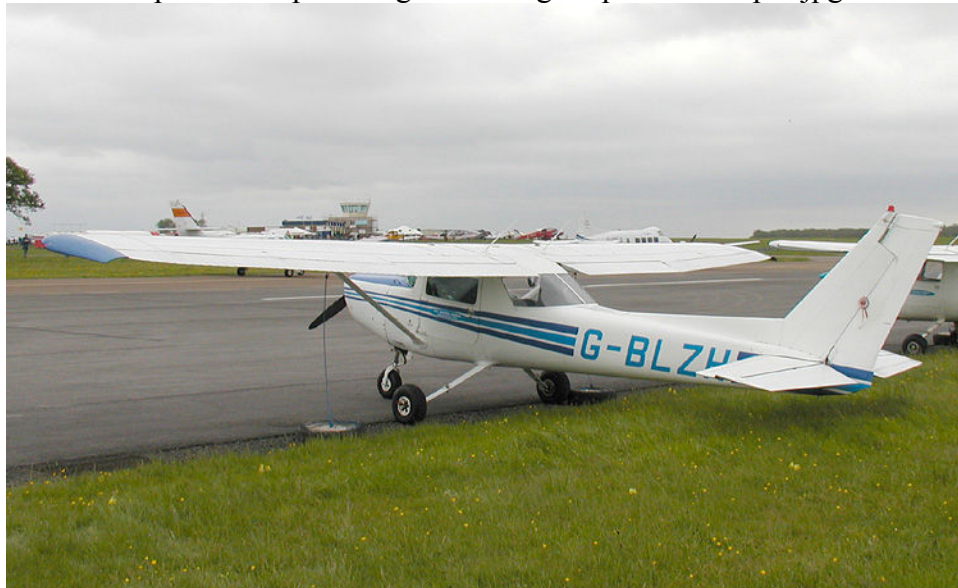
Figure 4 - Cessna Aircraft With Tricycle Landing Gear, Copied from the Public Domain at http://en.wikipedia.org/wiki/Image:Cessna.152.g-blzh.arp.750pix.jpg
