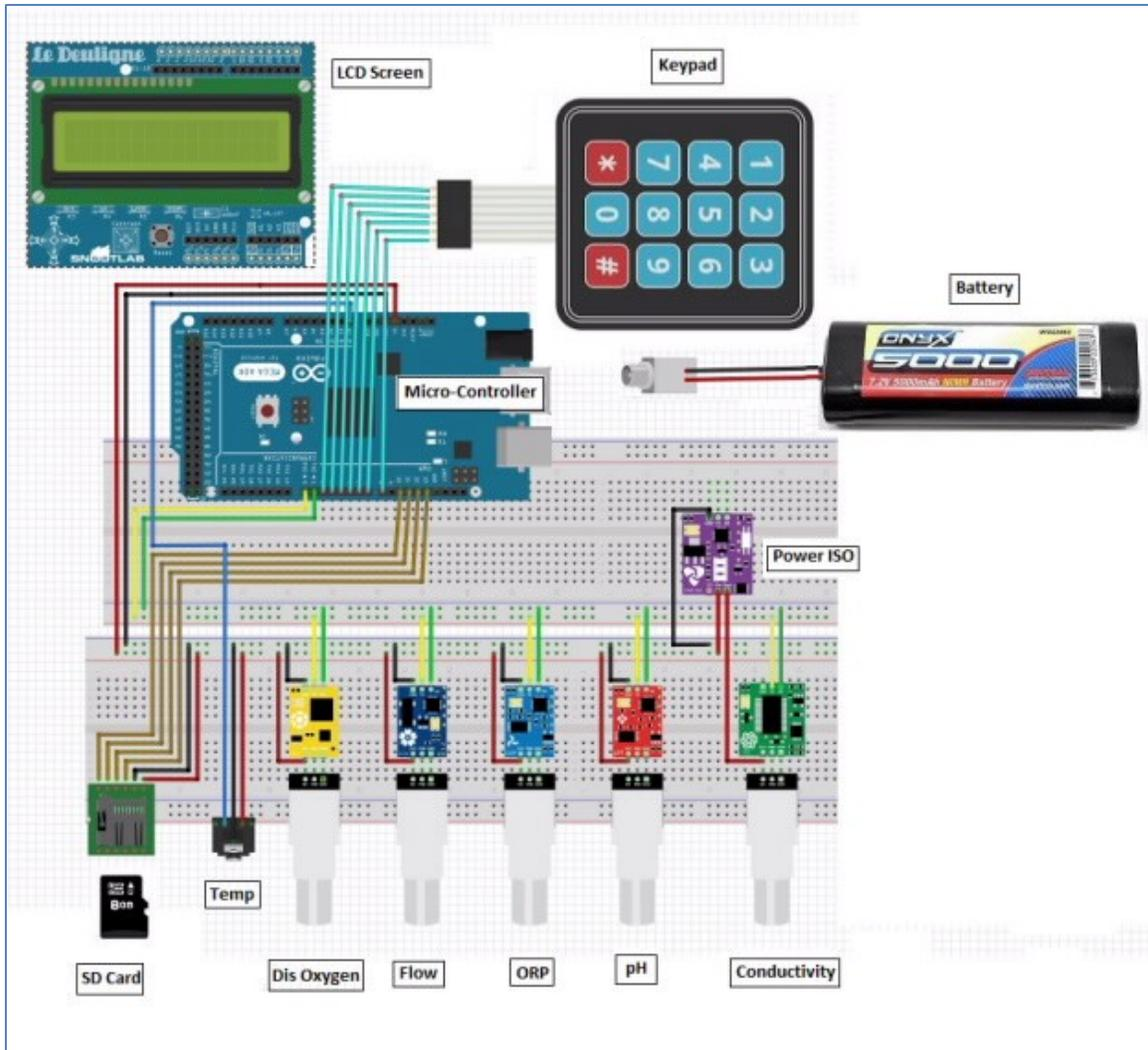
**Figure 2. Automated Multiparameter Water Quality Monitoring System**
