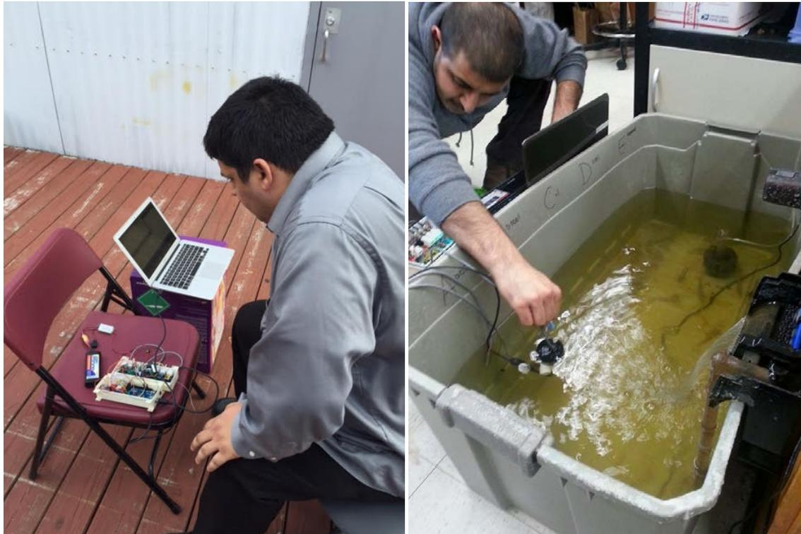
**Figure 3. Testing and Calibration of Automated Multiparameter Water Quality Monitoring System**
