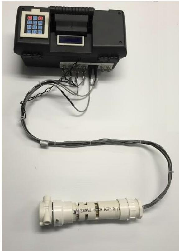
**Figure 5. Final Version of Automated Multiparameter Water Quality Monitoring System**
