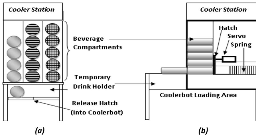
Figure 5 Cooler Station Showing (a) Front View and (b) Side View
