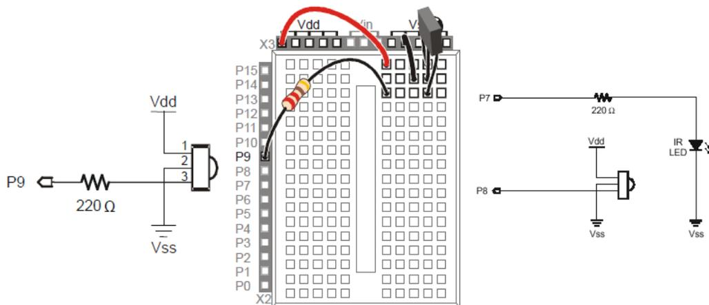
Figure 6 IR Circuits: Remote Control IR Receiver and IR Presence Sensor
