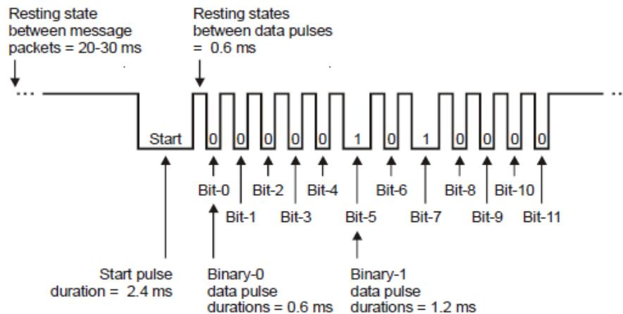
Figure 7 IR Message Timing Diagram
