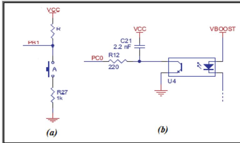
Figure 4 Digital I/Os circuit diagrams for (a) Pushbuttons and (b) Reflectance Sensor
