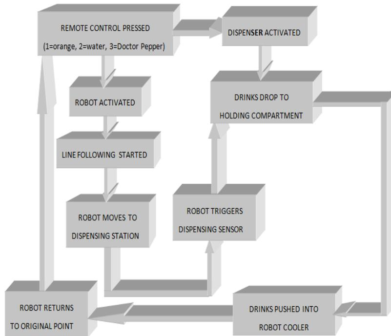
Figure 1 Block Diagram of Coolerbot Functionality
