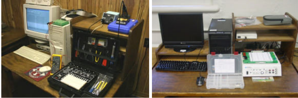
Figure 4: Workstation upgrades replaced electronic workbenches with NI ELVIS units
