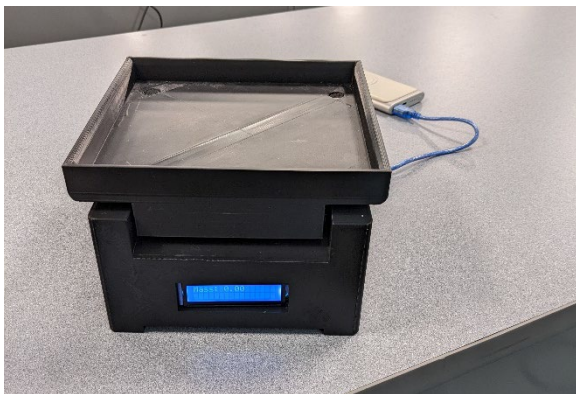
Figure 1: A balance utilizing a force sensing resistor in an enclosure
