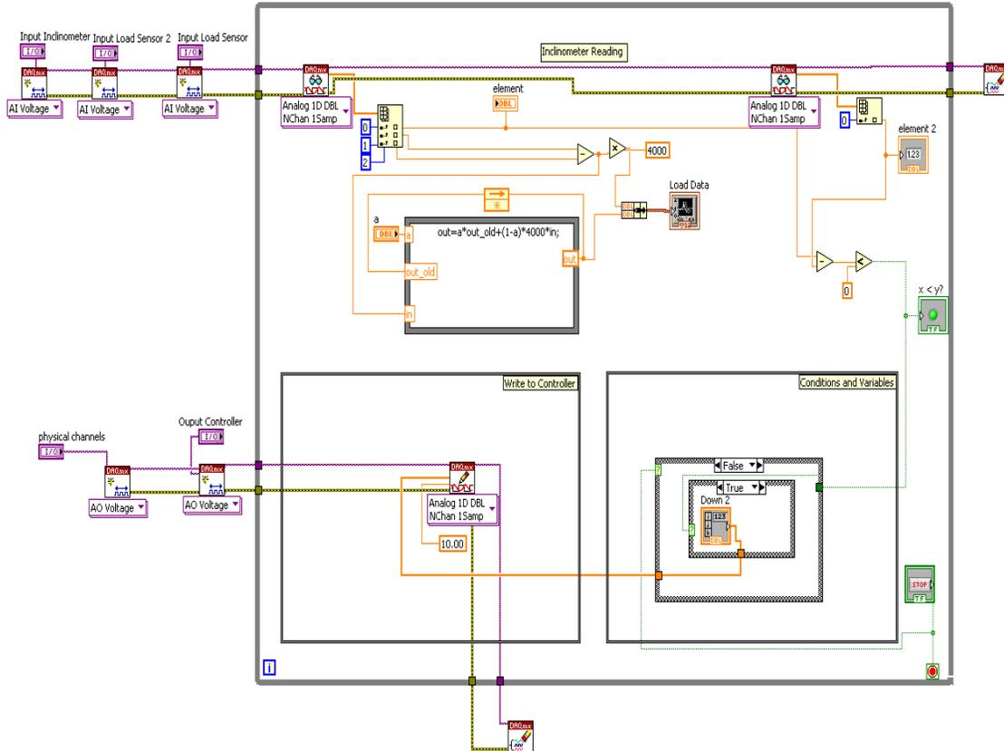
Fig. 3. LabVIEW front panel for pump jack control system
