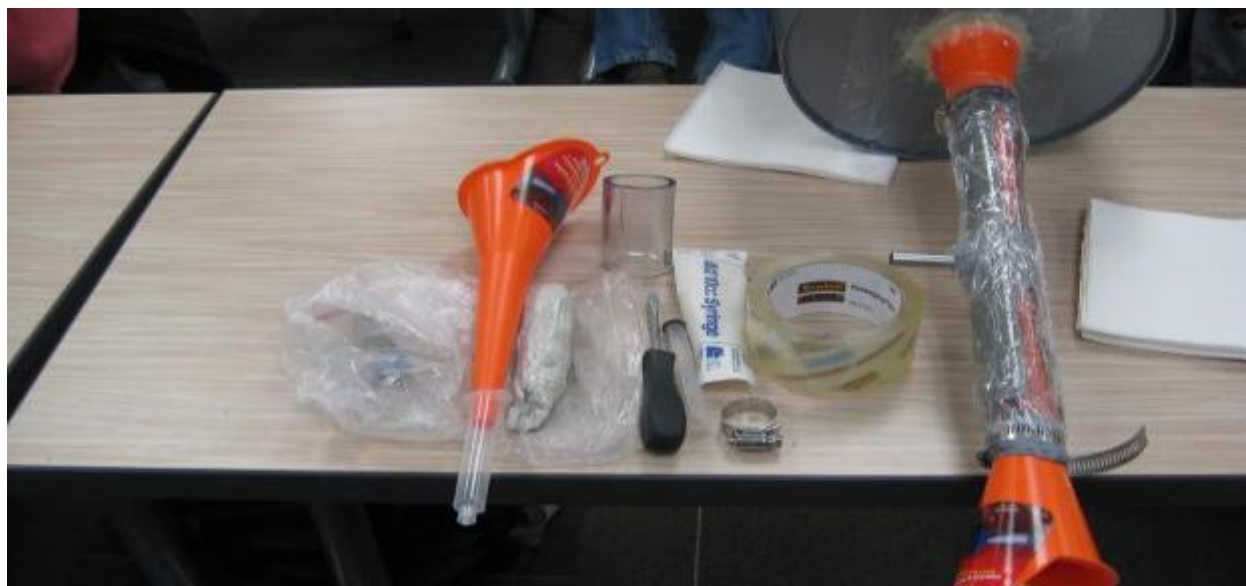
Figure 6. Supplies Used in Preparing a Funnel Venturi
