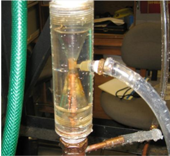
Figure 2. Photograph of Shop Fabricated Venturi
