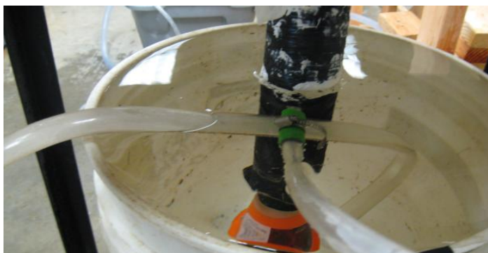
Figure 8. Close-up of Venturi Tap at the Throat
