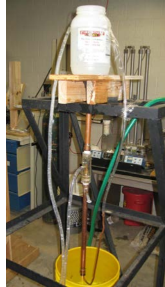
Figure 3. Flow System with Venturi Installed
