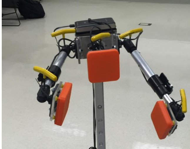
Figure 4. The adjustable head array with 3 buttons corresponding to moving a power wheelchair left, right and forward.
