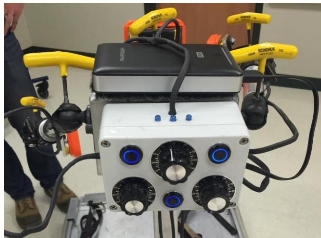
Figure 5. The controls for the adjustable head array. The dials adjust the force required to activate the switch and the lighted buttons indicate if the switch is active.
