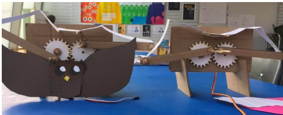
Figure 1: An owl and underlying mechanism - designs made by girls using FoldMecha, LocoTap microcontroller, and paper components.
