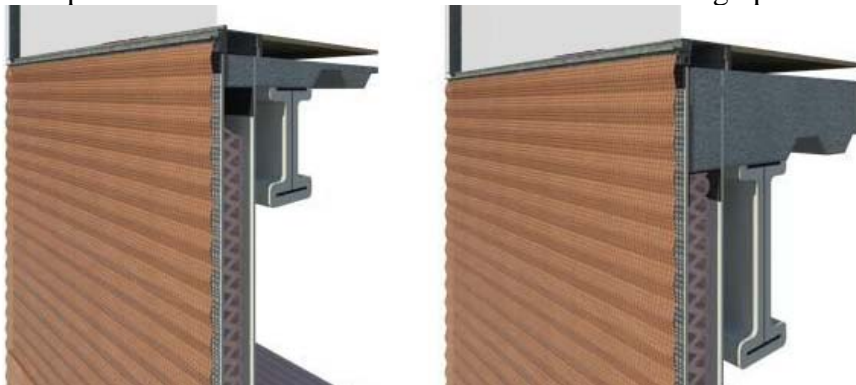
Figure 5 Analyzing parametrically-driven behaviors of element assemblies. A fully detailed beam at the slab condition with parametric control of the beam's depth and slab thickness. Remaining geometries follows spatial transformations of the beam and slab.(Alex Merlucci, NJIT)
