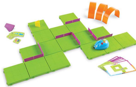
Figure 1: Learning Resources STEM Code & Go Robot Mouse Activity Set. This set includes a battery operated mouse that can be programmed to turn in four directions. The kit also include plastic maze grids and barriers for creating you own maze, suggested activity cards and double sided coding cards (see arrows in top left). This kit costs about $50 and the mouse alone costs about $20.
