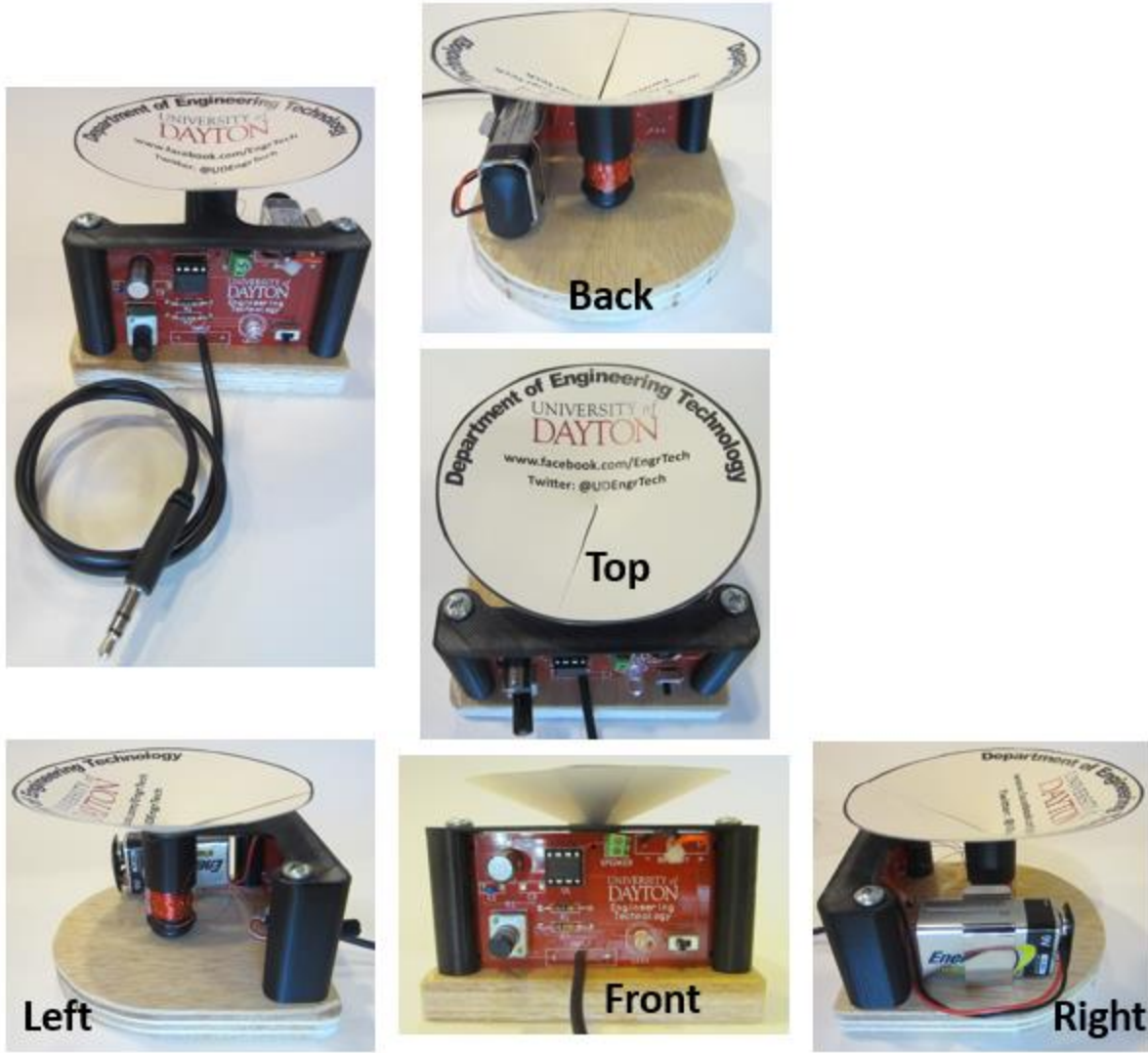
Figure 6. Views of Completed Assembly
