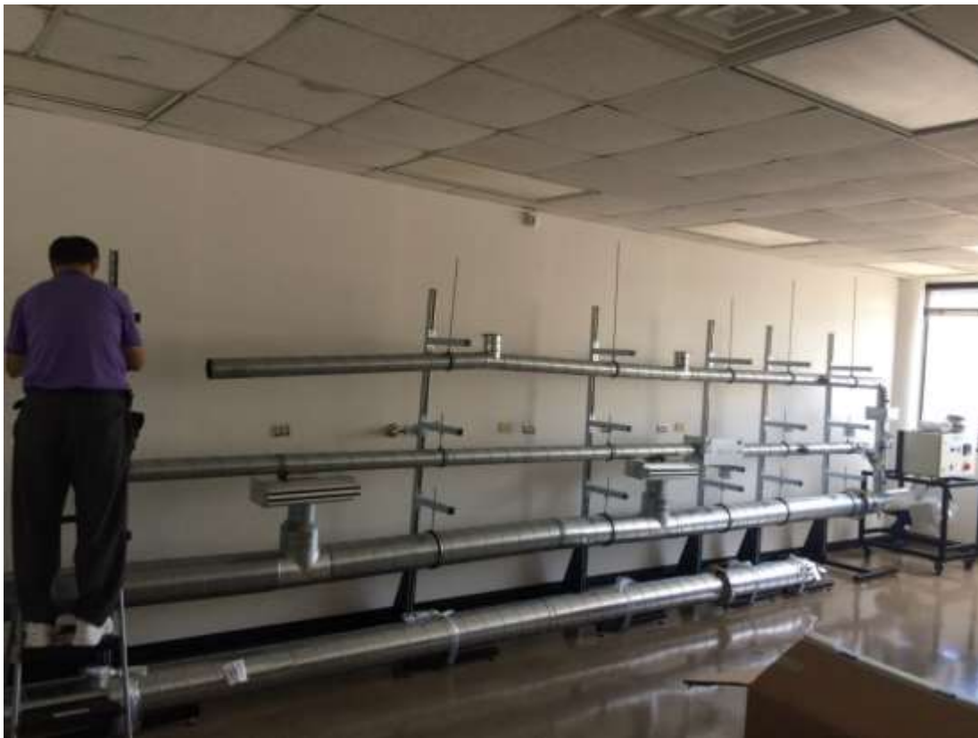
Figure 1. Thirty feet length space is needed for GUNT HL 710 Air Duct Systems installation.
