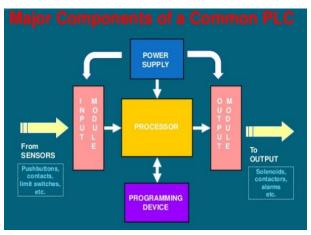
Figure 1. Major Components of a PLC
