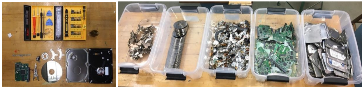
Figure 1: (left) The components of inside a waste hard drive. Disassembling work done by the students. (right) Sorted components after the sustainability module.
