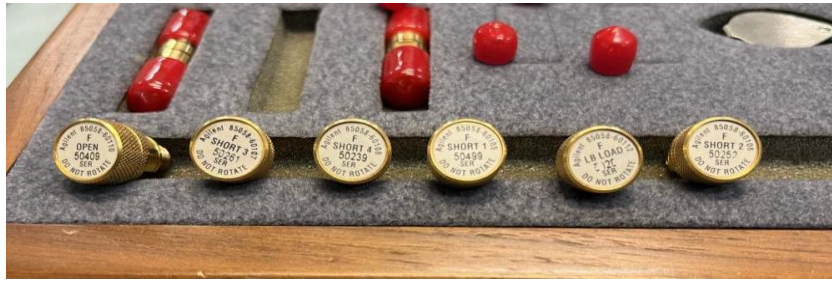
Figure 1: Mechanical standards within the calibration kit
