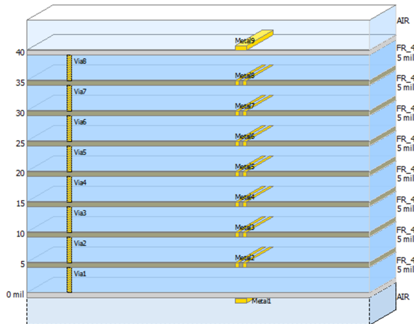
Figure 5. 9-layer PCB substrate model
