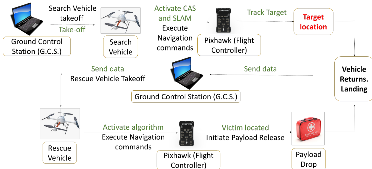
Figure 4. Overall architecture of the project for autonomous navigation of UAVs in indoor environments for search and rescue missions.
