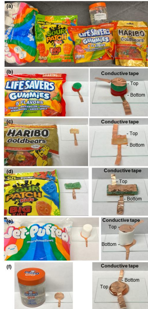
Figure 2. Materials and preparation with conductive tapes for capacitance measurement. (a) Five product packages used in this experiment. Three different types of gummy candies. (b) Life Savers. (c) Haribo Goldbears. (d) Sour Patch. (e) Jet-Puffed marshmallow and (f) Elmer's Gue glassy clear slime.
