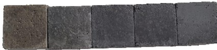
Figure 4: Cement mortars with 0, 0.5, 1.0, 1.5, 2.0% graphene
