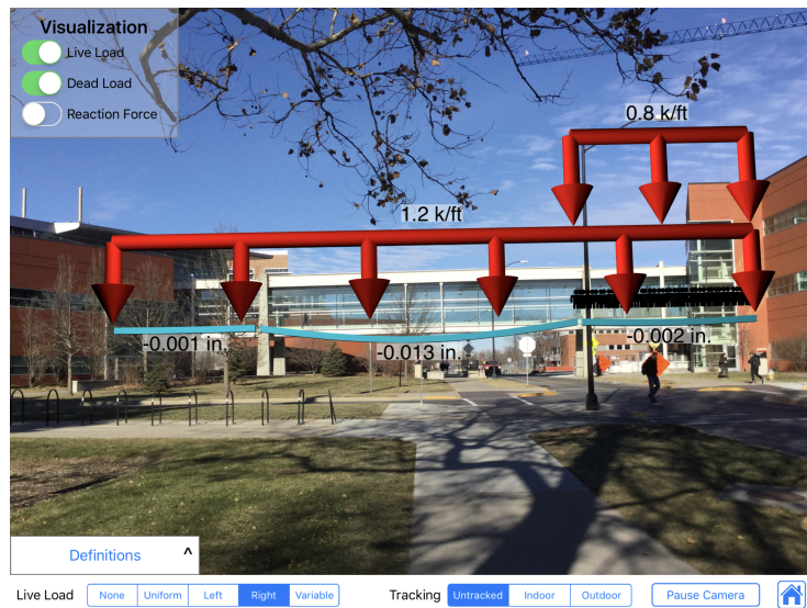
Figure 4: Unguided version of the current skywalk application, with enabled visualization of dead and live loading conditions.
