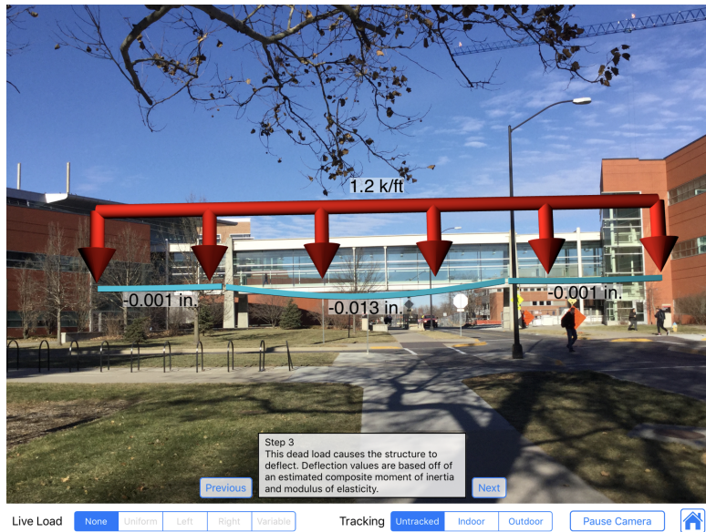
Figure 3: Guided version of skywalk application, with an example procedural step explaining deflection values.
