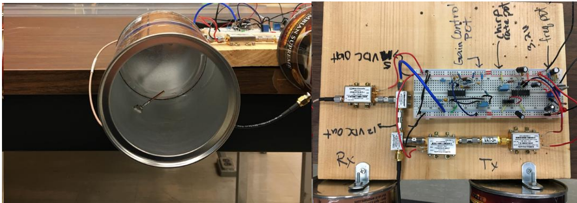
Figure 1. (Left) Coffee cans used as an antenna, (right) Physical layout of the radar system.
