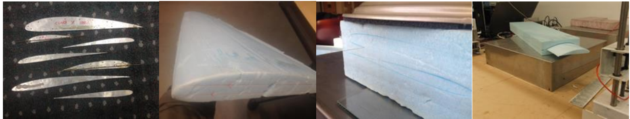
Figure 6: (Left to Right) Wing templates, wing section, wing section being cut, resultant wing shape
