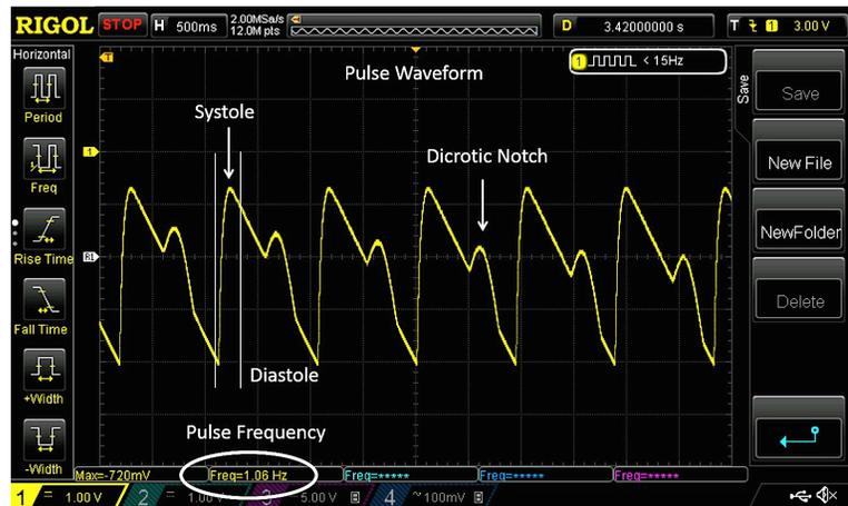
Figure 1: Output of PulseFit highlighting the cardiac phases.
