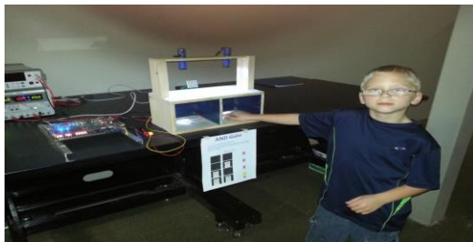
AND gate with one input (Right hand) LED matrix is off
