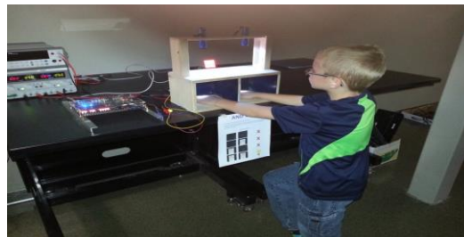
AND gate with two inputs (both hands) LED matrix is on
