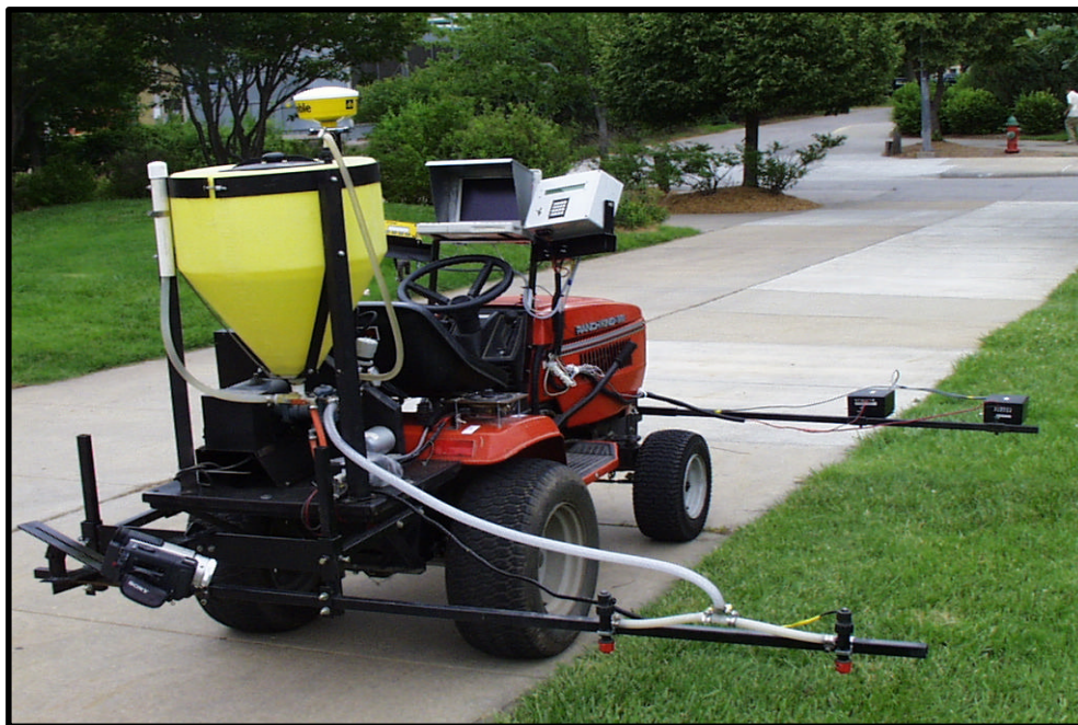
Figure 2. Weed detection system with variable rate applicator.
