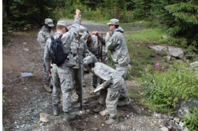
Figure 1. Dynamic Cone Penetrometer Tests at the McCullough Gulch Bridge Site
