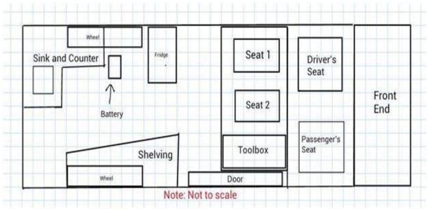
Fig. 1.1 Vehicle Schematic
