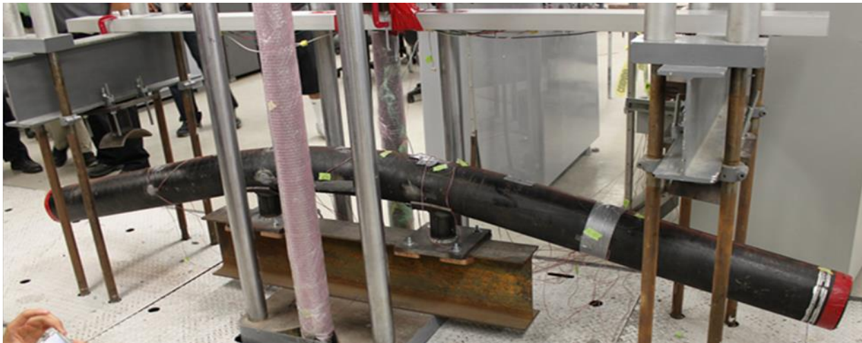
Figure 2 – Four-Point Bending Test of a Pipe
