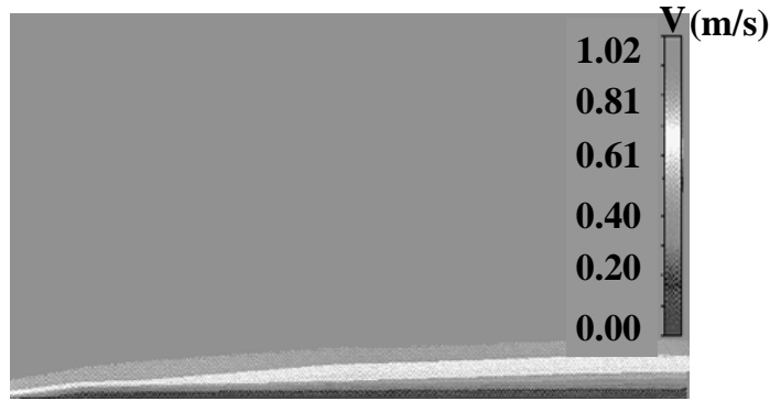
Figure 2. Velocity contours for the steady flow of water over a flat plate. The water approach velocity is 1 m/s.
