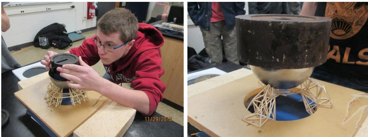
Figure 1. Sample trusses to hold a hemispherical metal shell. Additional static load can be added as shown. Instron universal testing machine is also used to find the exact ultimate failure load.
