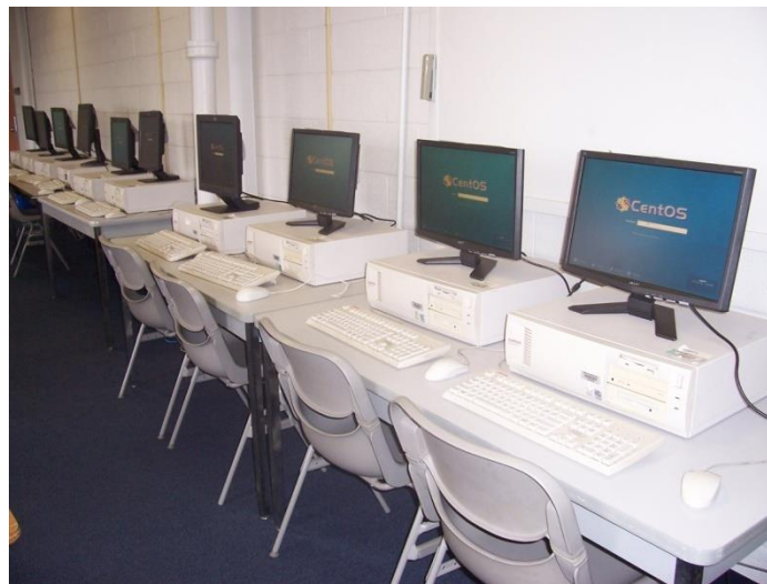
Fig. 2 A 10-node commodity cluster built of retired PCs
