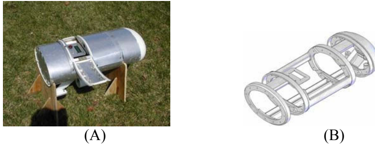
Figure 1: The first generation probe on dock (A) and the internal skeleton made from ABS plastic (B).
