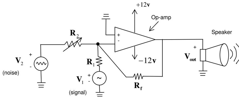
Figure 4: Signal-to-Noise Ratio Practical Exercise Circuit
