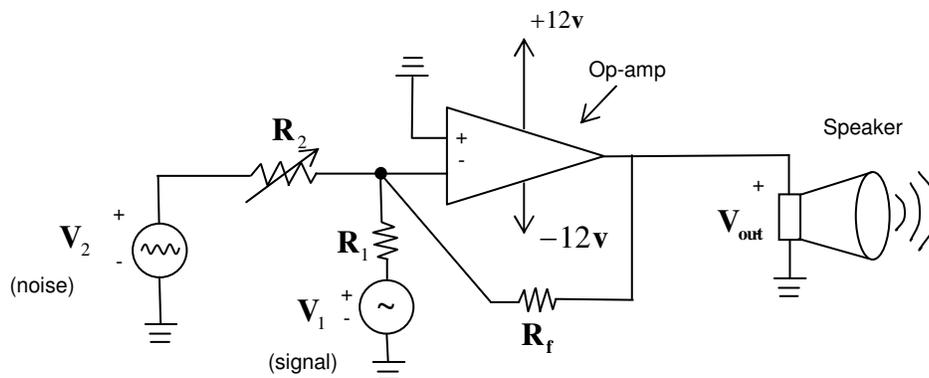
Figure 4: Signal-to-Noise Ratio Practical Exercise Circuit
